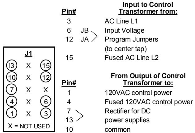
Figure 21: Connector J1 Pin Assignments
