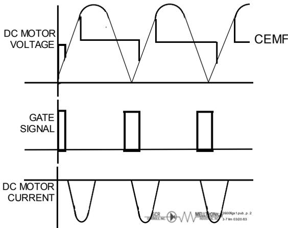
Figure 10: Voltage and Current Waveforms - Motoring Operation
