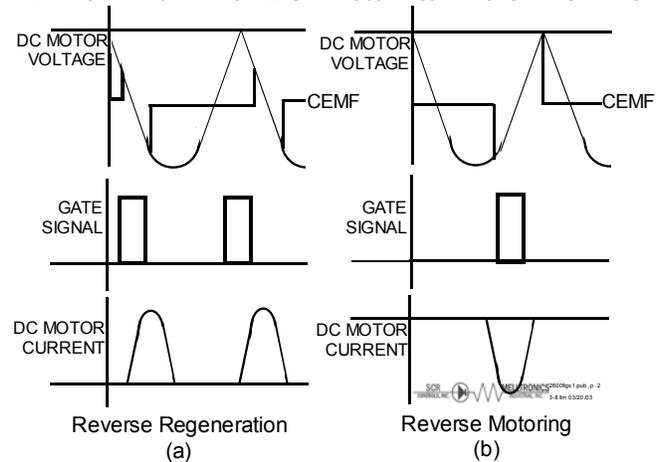
Figure 11: Voltage and Current Waveforms - Reverse Operation
