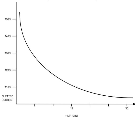
Figure 25: Inverse Time Trip Overload Characteristics
