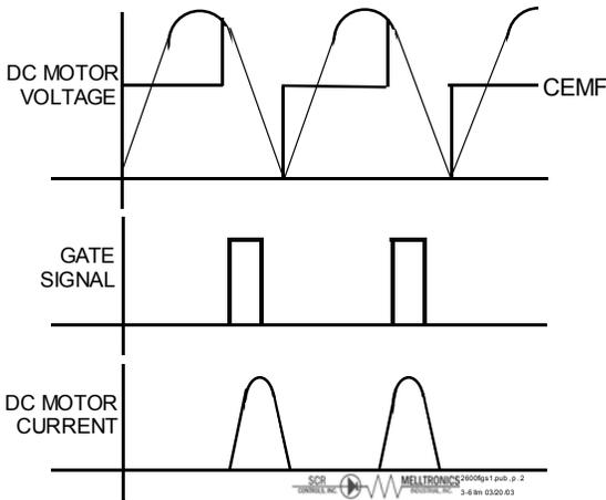
Figure 9: Voltage Current Waveforms – Motoring Operation
