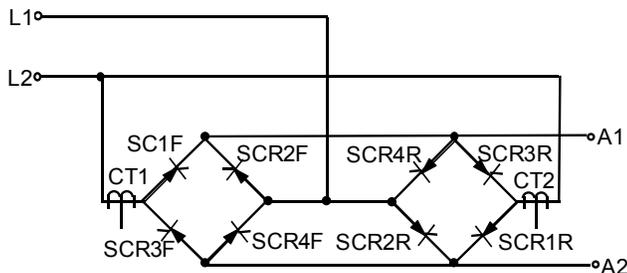
Figure 5: SCR Power Conversion Assembly
