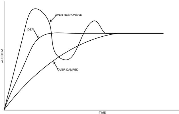
Figure 27: Stability Effects on the Velocity Profile
