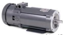
Integral DC Tach 1/4 - 5 HP Integral 50 V/1000 RPM DC Tachometer 90 or 180 Volt Armature 48 - 1810AT Frame
