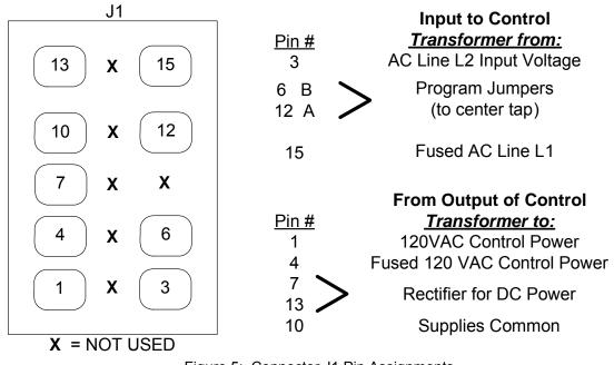
Figure 5: Connector J1 Pin Assignments
