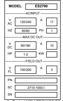
Figure 2: Typical MELLTRONICS ES-2700 Nameplate
