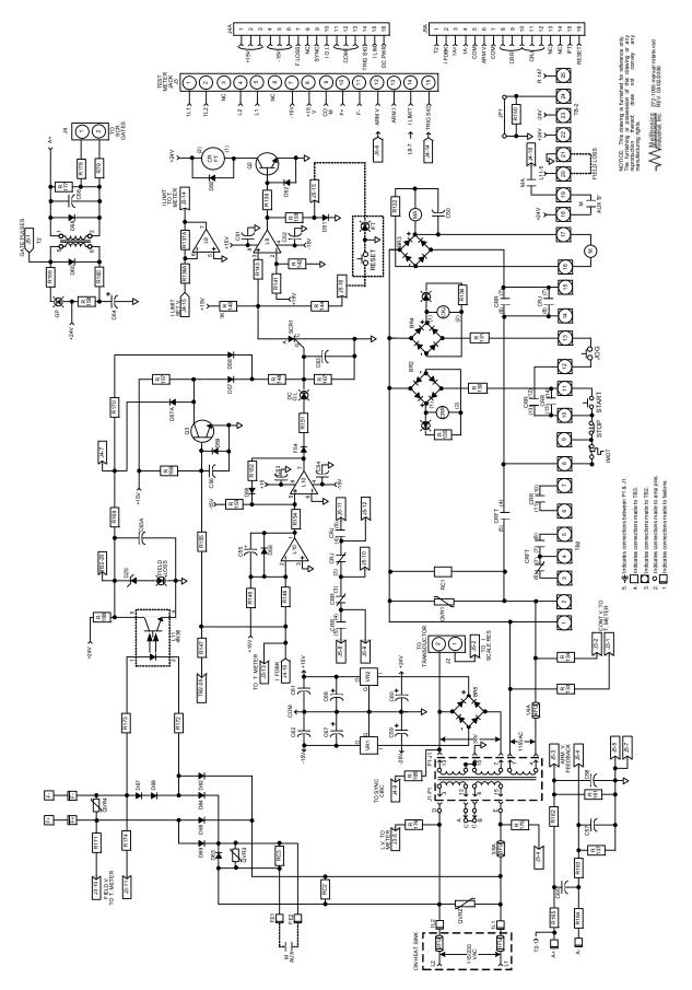
Figure 20: Bottom PC Board Schematic - Diagram 272-1005
