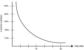
Figure 9: Inverse Time Trip Overload Characteristics
