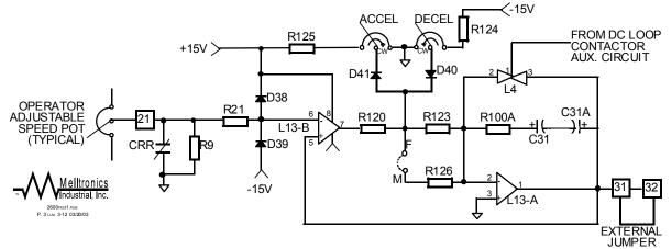
Figure 15: Accel/Decel (Reference Ramp) Circuitry
