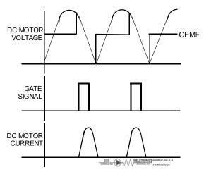
Figure 9: Voltage Current Waveforms – Motoring Operation
