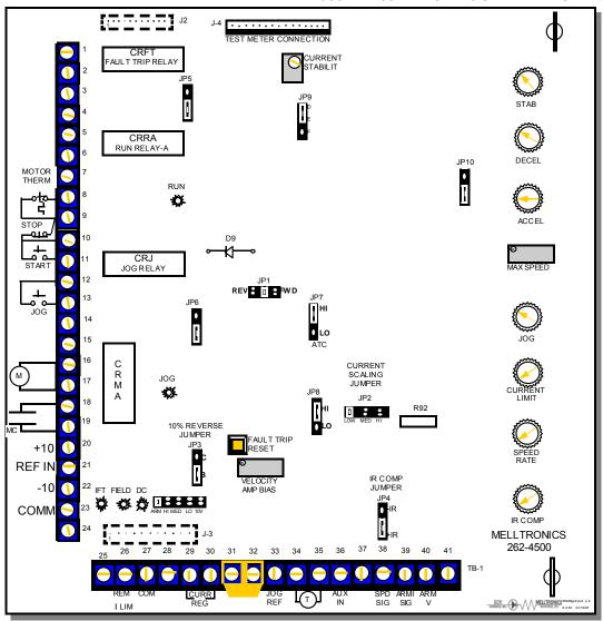
Figure 26: Upper Control Board Operating Features
