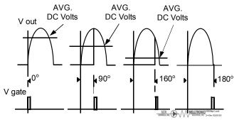
Figure 7: Typical SCR Voltage Waveforms
