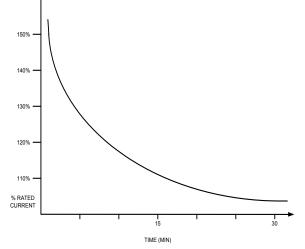
Figure 25: Inverse Time Trip Overload Characteristics
