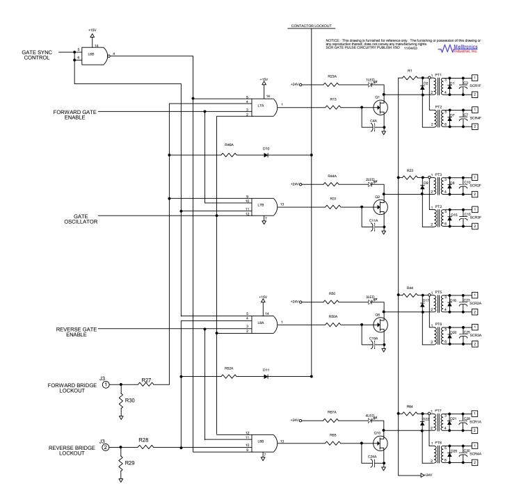
Figure 12: SCR Gate Pulse Circuitry
