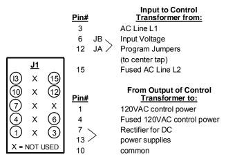
Figure 21: Connector J1 Pin Assignments
