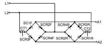
Figure 5: SCR Power Conversion Assembly
