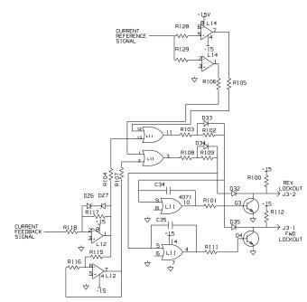
Figure 14: Power Bridge Lockout Circuits
