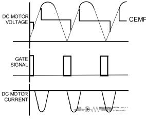
Figure 10: Voltage and Current Waveforms -Motoring Operation
